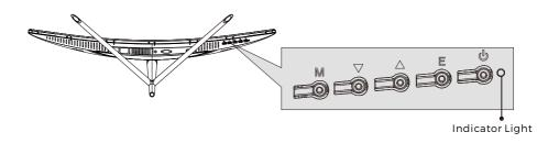
Solid blue light indicates power is on and the monitor is operating normally. Flashing blue light indicates no video source has been detected. Red light indicates that no horizontal or vertical signal has been detected or voltage is low. Please ensure your computer is on and all video cables are fully inserted and/or connected.
