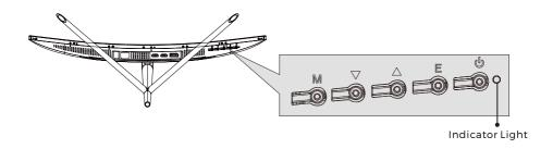
Solid blue light indicates power is on and the monitor is operating normally. Flashing blue light indicates no video source has been detected. Red light indicates that no horizontal or vertical signal has been detected or voltage is low. Please ensure your computer is on and all video cables are fully inserted and/or connected.
