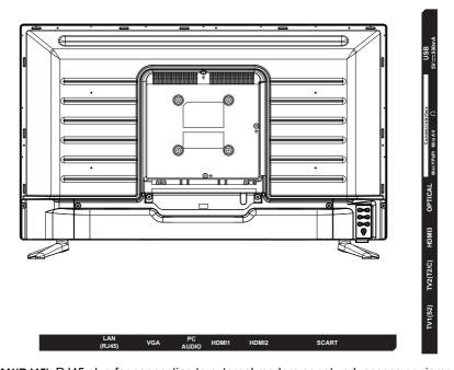
LAN(RJ45): RJ45 plug for connecting to external modem or network access equipment.
