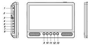
1. POWER ON/OFF 2. CARD SLOT 3. USB 4. HEADPHONE OUT JACKS 5. AV OUT 6. AV IN 7. DC OUT 8. DC IN 9-12V 9. UP/ Prev 10. DOWN/Next 11. SOURCE 12. ►II(PLAY/PAUSE) 13. ■ STOP 14. DC IN 15. AV IN 16. HEADPHONE OUT JACKS 17. POWER ON/OFF 18. UP 19. DOWN 20. MODE 21. LEFT /VOL-22. RIGHT/VOL+
