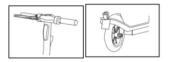
Press the key  $(\Phi_{di})$  to turn ON the power, the headlights and taillights always be ON. Press the key  $(\Phi_{di})$  to turn OFF the power, the headlights and taillights go out.
