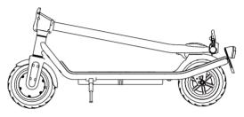
2) Right index finger lift the buckle lock up. Push the folding wrench outward with the thumb to put down the upright pole.
