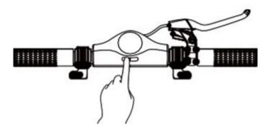
2. You have to manually moving the scooter with one foot on foot pedal and other foot kicking for speed. When you have achieved approximately 6km/h of speed then you push accelerator to start motor and for gaining more speed.
