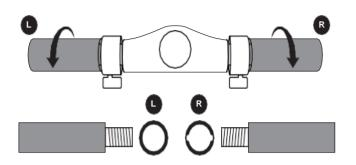
Please make sure to differentiate the left and handles carefully before installing the handles.
