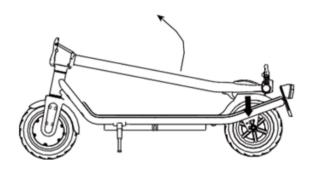
3) Raise the front pole and the pull up the folding wrench towards the upright pole and force it to lock.
