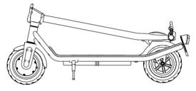
2) Right hand presses down the rear fender and left hand pulls up the long pole until folding hook gets out of the hook.
