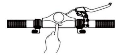
5. For safety, the rear drum brake must be used when driving at high speed. Use the right hand brake on the steer.
