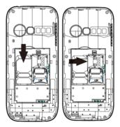
**Insert a memory card:** In order to use media player functions, a micro-SD memory card is required (not included in the package). The card must be placed into the SIM1 slot on the left inside the rear of the phone. Insert the micro-SD card as below shown,
