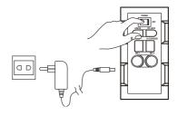
It is recommended to charge the battery about 6 hours before you start using the unit for the first time.
