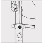
Press adjustment marble with one hand and adjust the telescopic rod to the proper position with the other hand. Users must adjust the height of the product to the proper position to ensure safe driving.
