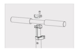
Use the screwdriver to lock the handle block.
