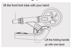
Lift the folding handle up with one hand and lift the front fork tube with the other hand and you hear a "click".
