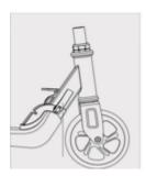
Press the folding lock firmly (the folding lock can adjust the tightness).
