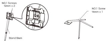
4. Insert the stand's plate into the opening on the back of the monitor. It should click into place. Make sure the stand is securely attached to the back of the monitor then remove the monitor from the remaining foam section and stand it up on a table or desk as desired.
