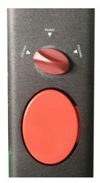
Press the red button to fold or unfold the e-scooter.
