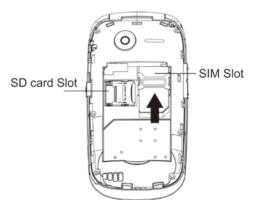
Inserting a memory card: in order to use camera and media player functions, a micro-SD memory card is required (not
