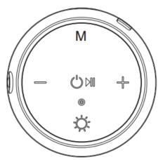
Light flash when on mode (full color sine move up and down) press 1st mode 1(Multicolor Rotating combination of graphics) press 2nd mode 2 ((two color conversion with double line) press 3rd mode 3 (light off) press 4th mode 4(light off) press 5th mode (one color move up with light bar ) press again light back to default status. ight mode button:
